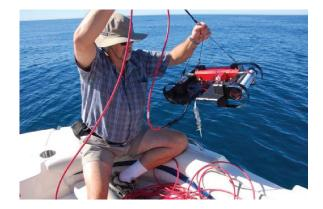
C-OPS is so lightweight it can be hand deployed, so the system can be operated from either small or large vessels. In addition, its free-fall system precludes any influence from the shadow of the ship.
